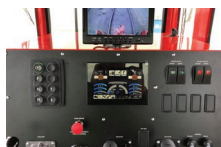
180-degree rotating console with a multifunction display. Dual four-way air suspension seats for operation from either side of cab when in rail mode.
