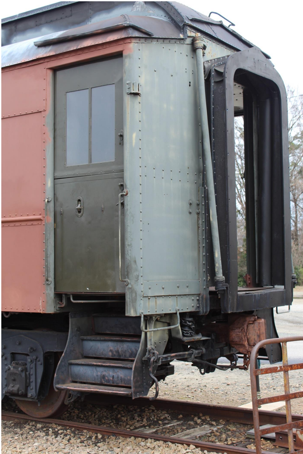
Dutch door in the closed position on the Men's room end of the car. All Dutch doors are similarly restored.
