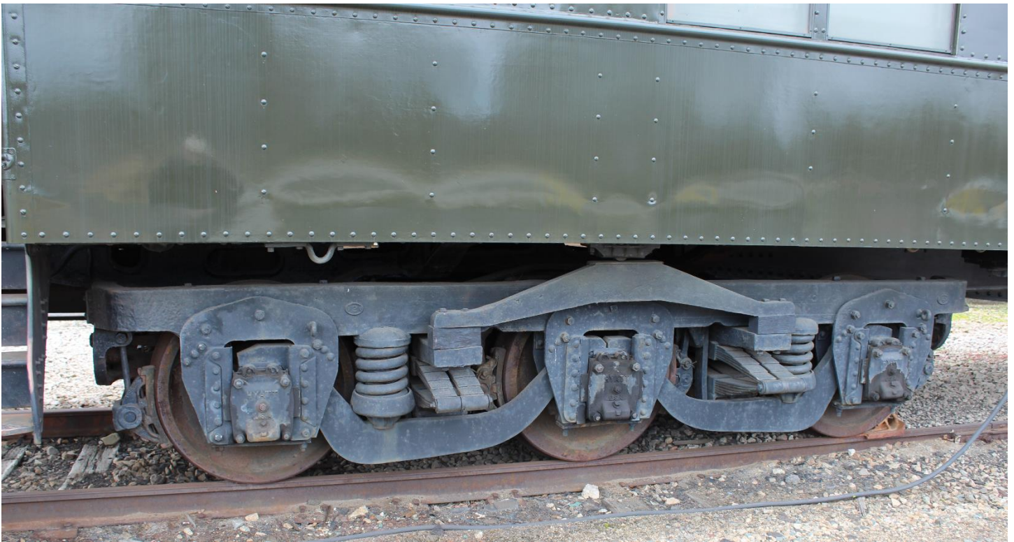
Truck Assembly – Men's room end. Friction Bearings replaced with Hyatt roller bearings in 2000.
