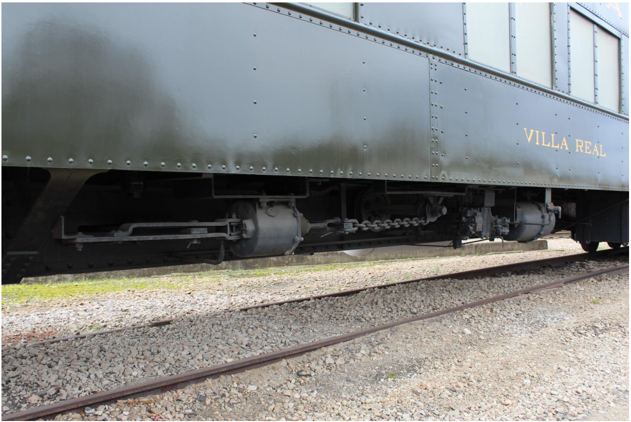
12" single brake cylinder, ABD break valves and reservoir.
