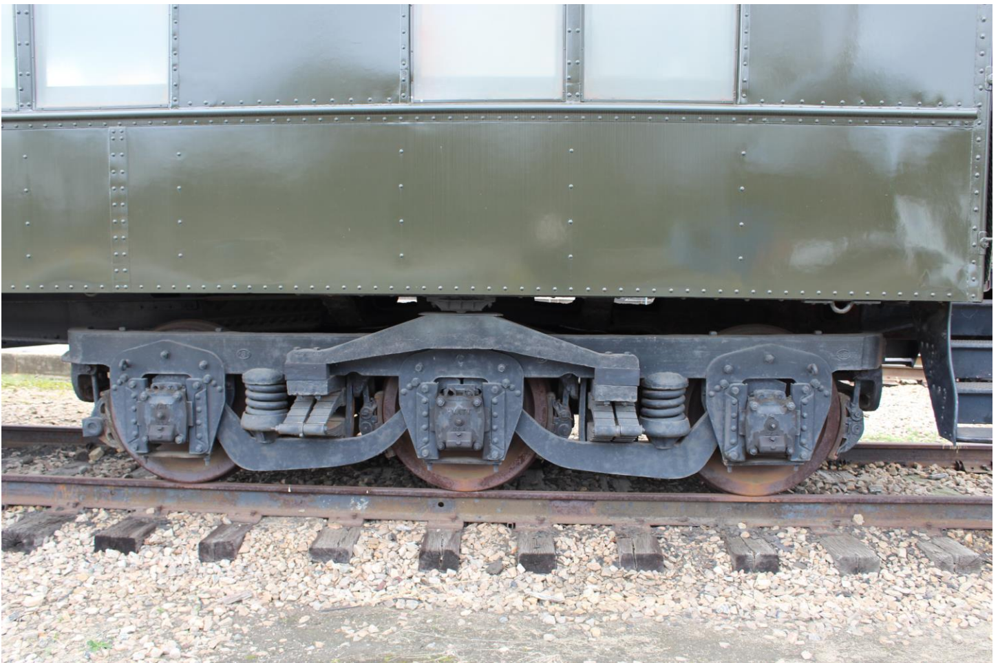
Truck Assembly under the Ladies Room end.
