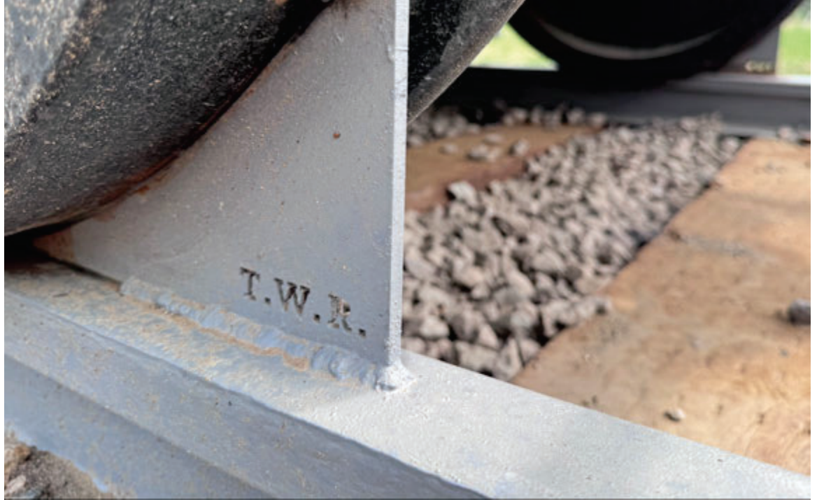
(Detail showing welded connection between wheels and train tracks of The Louisville Caboose. Applicant had these pieces laser cut with each his children's initials as shown above)
