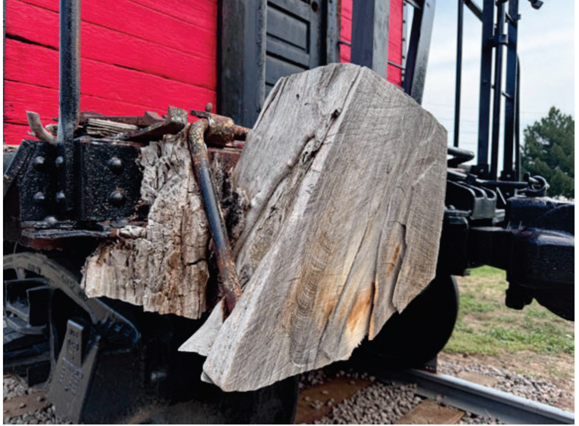
(Platform on South side of The Louisville Caboose showing the remnants of the trunk of a tree that had grown around the corner of the caboose while it was at Main St. & South Boulder Rd. location)
