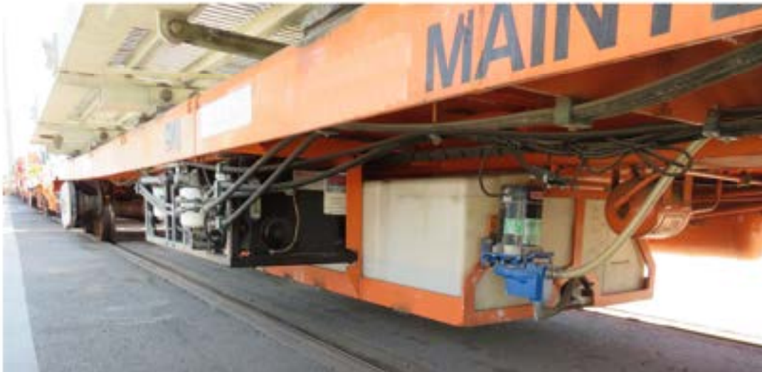
Pictured: Standard water pump/tank & hydraulic system
