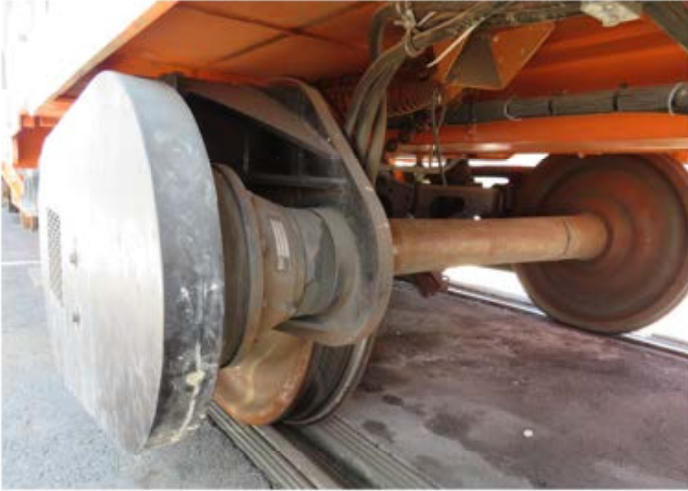
Pictured: Black Bruin hydraulic powerdrive motor for flatcar self-propulsion
