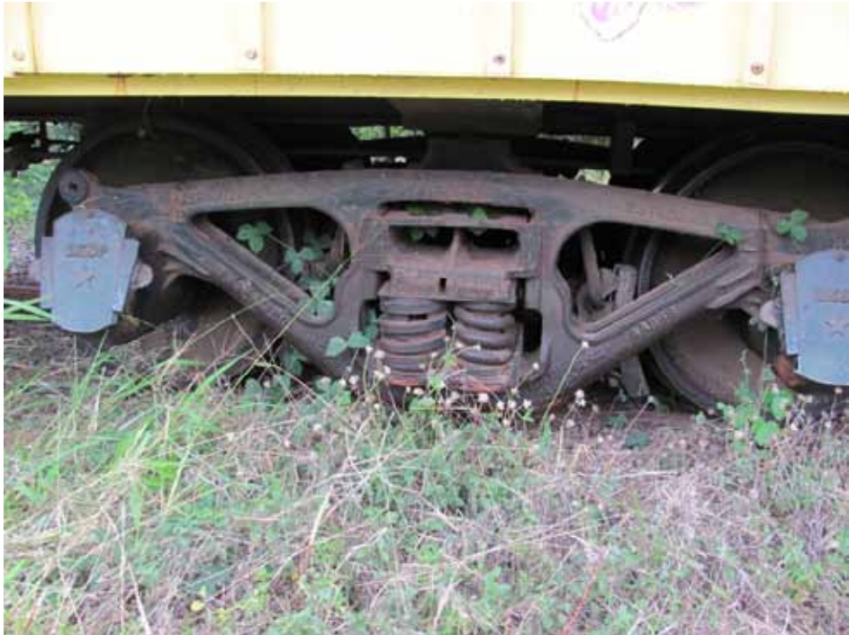
Coach 107 - Narrow Gage Freight trucks as applied to newer cars 105-109
