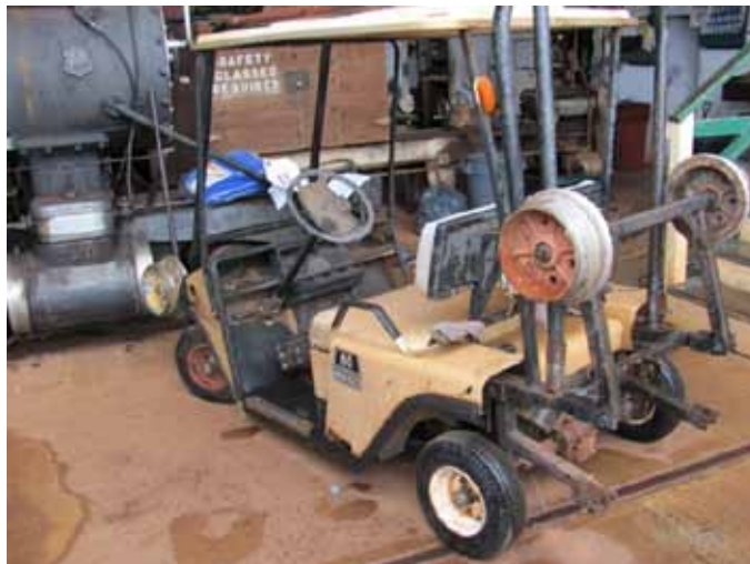
Track inspection vehicle converted from Golf Cart
